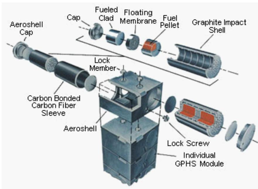
GPHS modules stand approximately two inches tall and have a base that is almost square with sides less than four inches in length. Each GPHS module is designed to weigh no more than 1.44 kilograms and produces a nominal thermal power of 250 watts at beginning of mission. A total of 18 modules are stacked together to provide the heat source for each of the radioisotope thermoelectric generators used on the Cassini mission.
